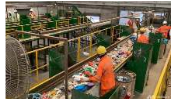
The Recyclables are placed on conveyor belts for manual sorting according to material types; paper, plastic, metal, glass etc.
