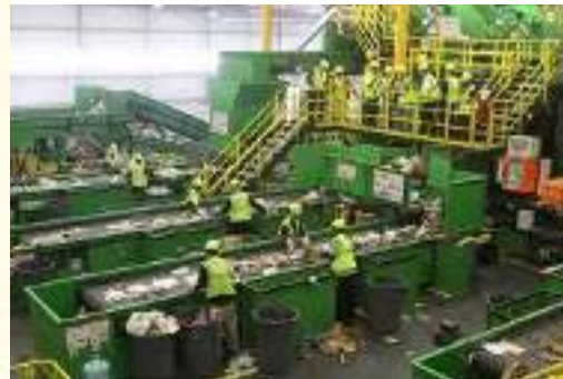
The Recyclables are placed on conveyor belts for manual sorting according to material types; paper, plastic, metal, glass etc.
